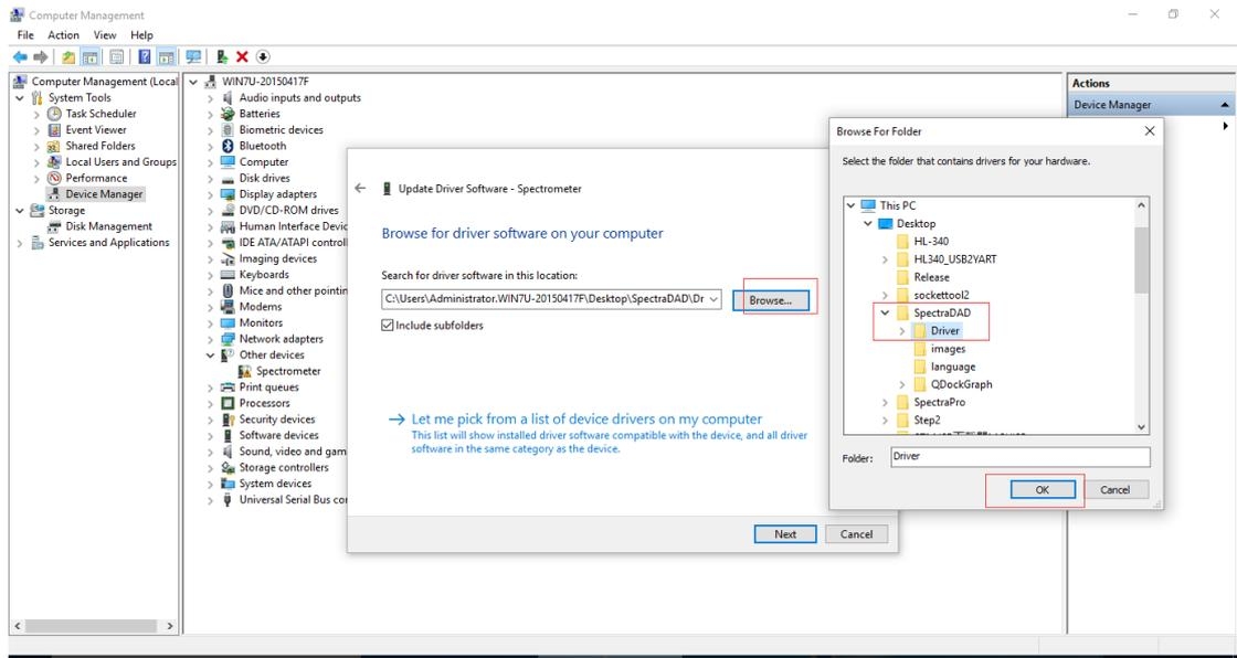
The driver files is located in the folder “**Driver**” after software installation.
